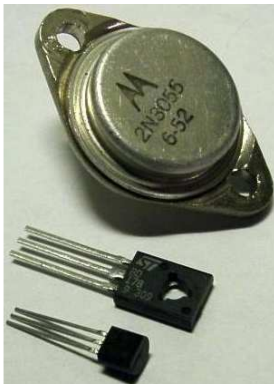
△ Fig.5.9 Enkele gangbare TO-behuizingen. Bron: World Wide Web
