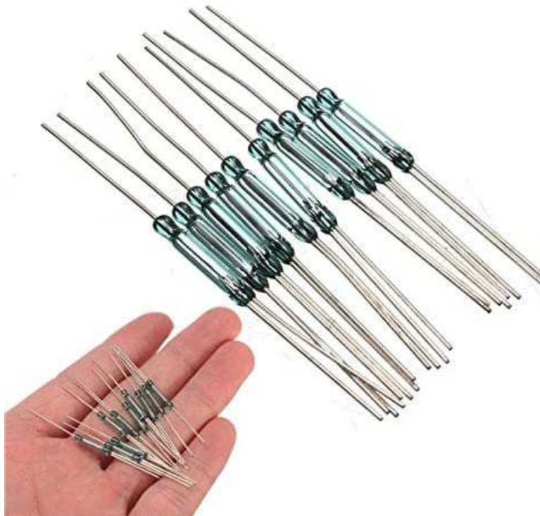
△ Fig.2.20 | Goedkope reedcontacten in glazen behuizing. Bron: World Wide Web
