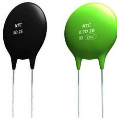
△ Fig.2.36 | Koppeltje NTC-thermistoren. Bron: https://www.electrical4u.com
