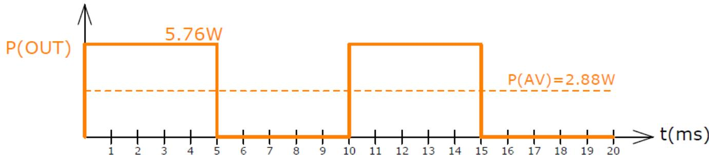
$$P_{RL} = V_{RMS} * I_{RMS}$$
