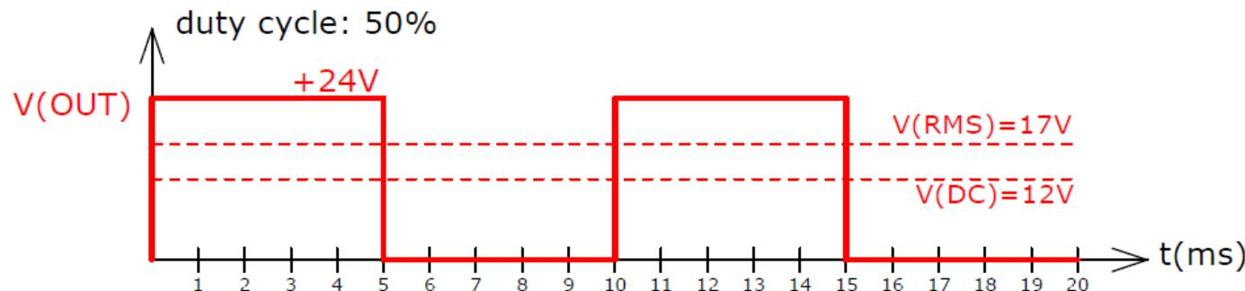
$$V(\text{OUT})_{\text{DC}} = 0,5 * 24 \text{ V} = 12 \text{ V}$$
