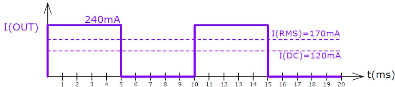
$$I_{DC} = \delta * I_{MAX} = 0,5 * 240 \text{ mA} = 120 \text{ mA}$$
